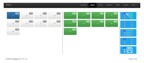
The left side of the long string is input area: GMS0909 will have 9 buttons, GMS1818 has 18 buttons, GMS3636 will have 36 buttons. The right side is output area, the buttons are the same with input area. And there're 5 buttons: The 1<sup>st</sup> for 1 to all, 2<sup>nd</sup> for 1 off to all, 3<sup>rd</sup> for 1 to 1, 4<sup>th</sup> for all off, the last one is for scene save and recall. (Change names can be done in Caption interface)
