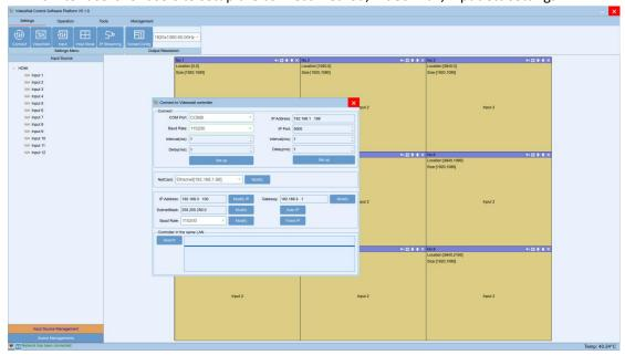
Connect is for users to setup the communication methods for the control PC and the controller, users can set up the COM and IP address those parameters here. After modified the parameters, will need to reconnect and restart the controller.
