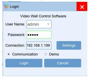
To click "Settings" login, it will be showing below interface, users can set up the LAN(IP) or the COM(RS232) as below, the default IP address is 192.168.1.199, and the baud rate is 115200.
